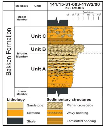
Figure 2: Stratigraphic chart showing the type-section geological makeup of the Bakken Formation in Saskatchewan
